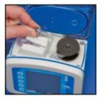
Grasp black ring retainer, gently wrap tubing around rotor, insert retainer directly into right pocket. DO NOT OVERSTRETCH TUBING.
